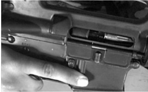
Figure 3-15. Brass Obstructing the Chamber.
